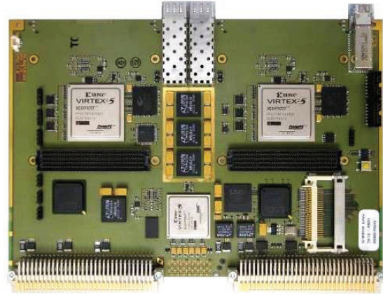
Figure 6: Digital Back-End FPGA Signal Processing Board Prototype [4]. The two large Virtex-5 FPGAs receive the ADC data from the digitizer mezzanines (via adjacent 500-pin connectors, mezzanines removed on photo).
