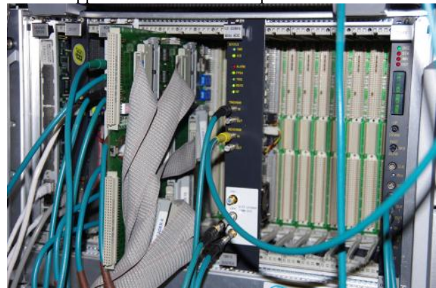
Figure 4: 18K10 in the VME subrack. VME extension left to the 18K10 is used to monitor the VME bus timing using logic analyser.
