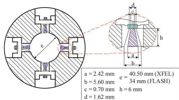
Figure 1: Cross-section of the cone-shaped pickup [5].
