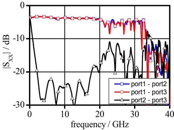
Figure 5: Transmission coefficient of the combiner ATM 213H.
