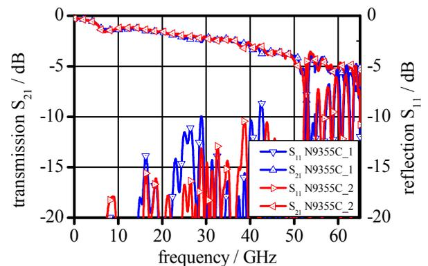
Figure 4: Transmission coefficient for the limiters Agilent N9355C.
