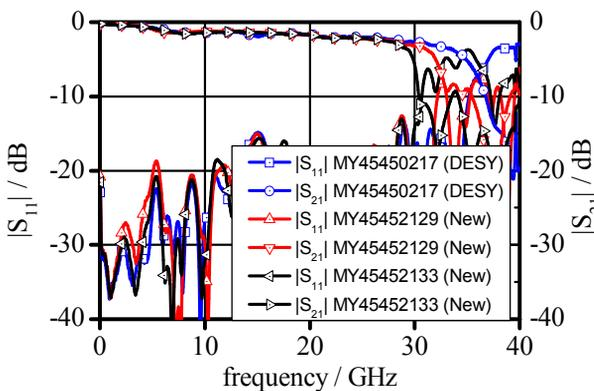
Figure 6: Transmission coefficient for Agilent N9356 limiters.
