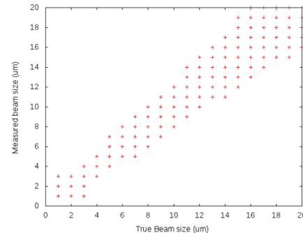
Figure 5: Calculated 1- $\sigma$  statistical resolution contours for 47-element CA with  $5 \mu\text{m}$  elements at the ATF2 with 1 nC bunches.
