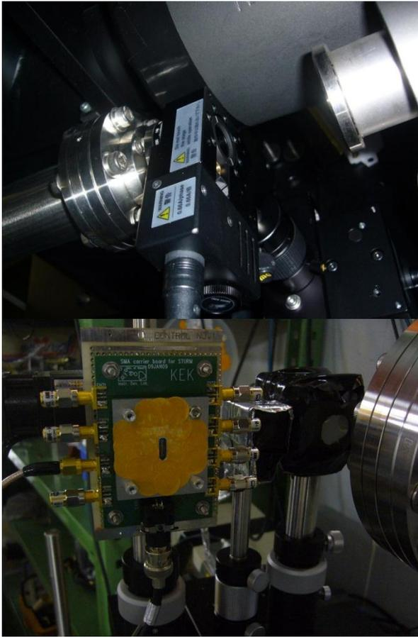
Figure 3: Rotating mask holder (above), and detector on rotating stage (below). Next to detector are a PMT with Ce:YAG scintillator and a CCD for initial alignment.
