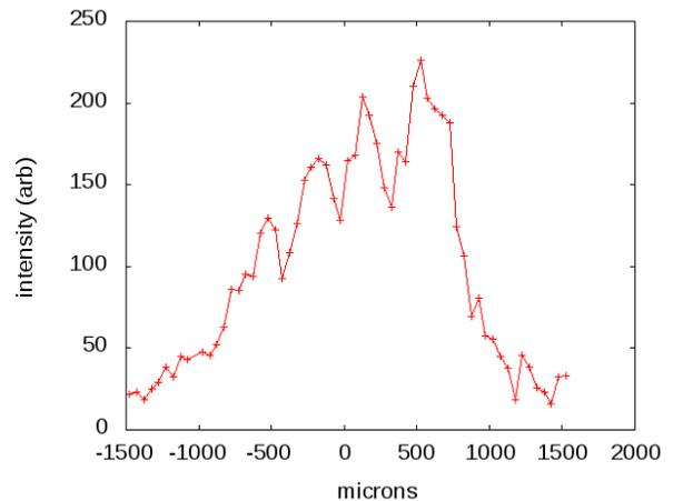
Figure 7: Pre-tuning scan, corresponding to about 15 micron beam size (hand fit).
