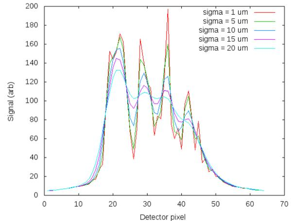
Figure 4: Simulation of expected beam patterns for 50-micron pitch detector at different beam sizes.
