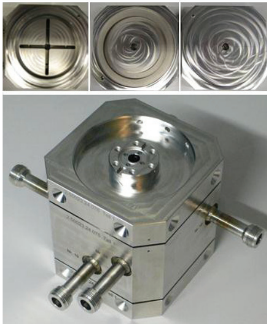
Figure 4: SwissFEL undulator prototype: pictures of the 3 parts composing the pickup body and final assembly after brazing.
