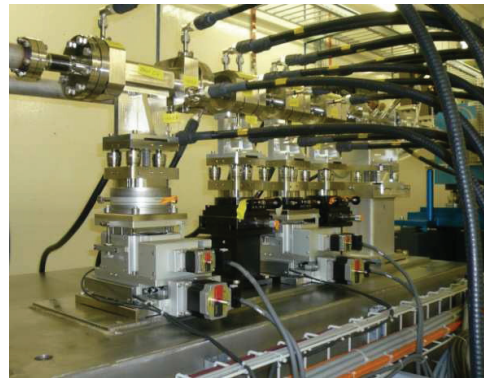
Figure 8: BPM test array at SwissFEL 250MeV test injector facility.
