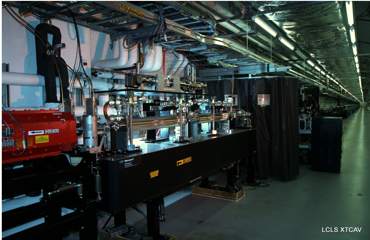
Figure 3: Photo of the XTCAV installed at the downstream end of the undulator beamline.
