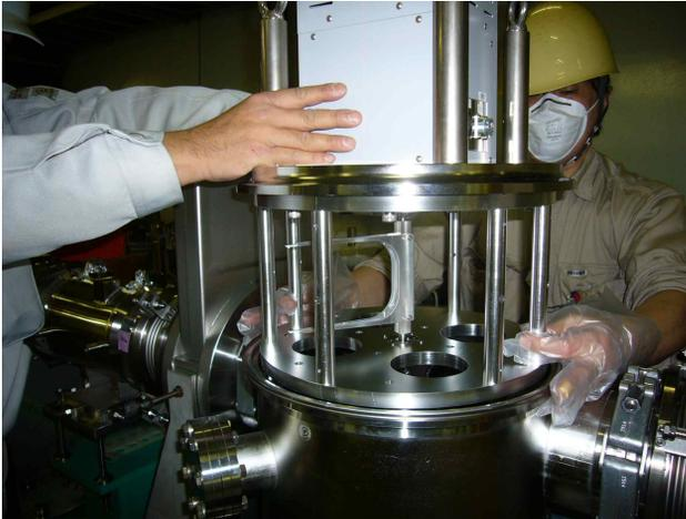
Figure 2: Installation of the horizontal flying wire monitor.
