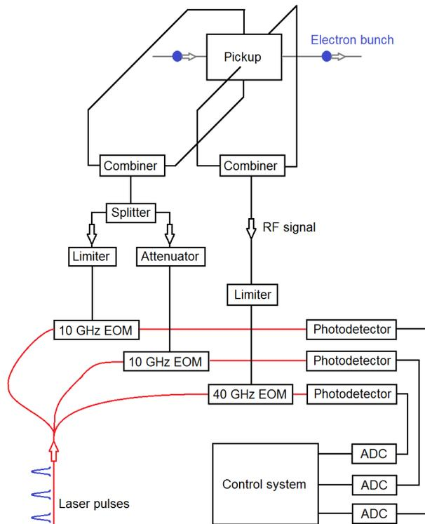
Figure 1: Schematic design of the BAM system.
