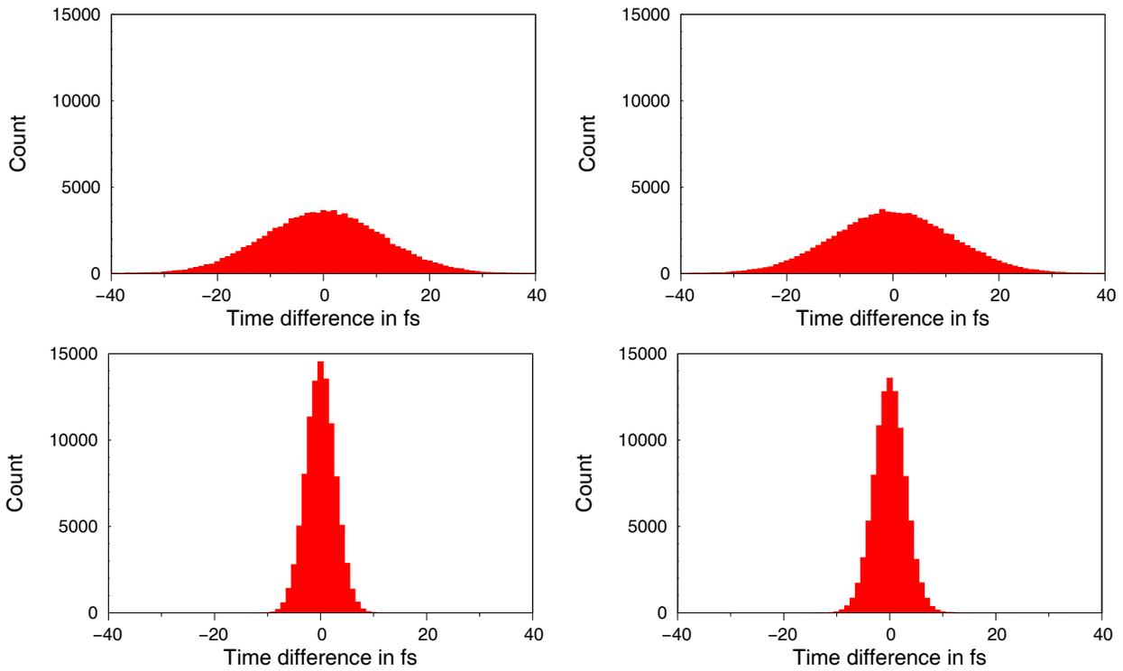
Figure 4: Count of the difference between  $t_{\text{bunch}}$  and  $t_{\text{sim,meas}}$  for different settings. The bunch charge is set to 20 pC in the top row and to 200 pC in the bottom row. The timing jitter of the bunch is set to 25 fs in the left column and to 100 fs in the right column.
