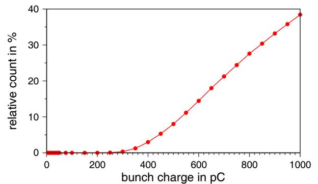
Figure 7: The working range of the EOM for detecting the correct timing is limited by  $\frac{1}{2}U_{\pi,\text{RF}}$ . The graph shows the relative count with  $U_{\text{RF}}$  higher than  $\frac{1}{2}U_{\pi,\text{RF}}$  for different bunch charges by using a timing jitter of 100 fs. For bunch charges higher than 200 pC the 10 GHz EOM has to be used as the fine channel for measurement of the timing shift.
