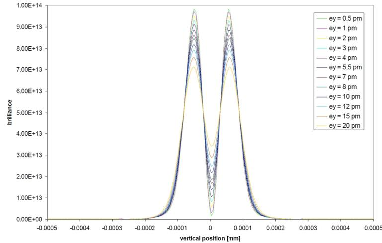
**Interferometer Branch – Emittance Resolution**
