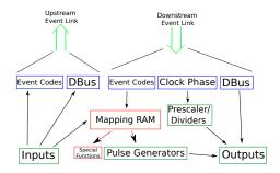
Figure 3: Logical connections inside an EVR
