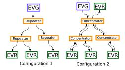
Figure 1: Two system configurations for the MRF Timing System
