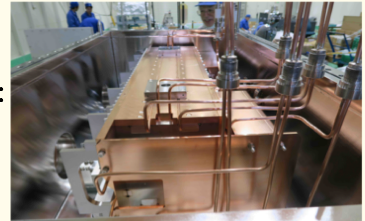
Septum magnet for injection.
