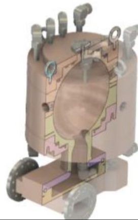
New pulse compressor Spherical-Cavity Pulse Compressor (SCPC)
