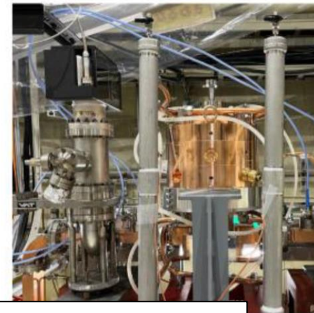
New pulse compressor Spherical-Cavity Pulse Compressor (SCPC)
