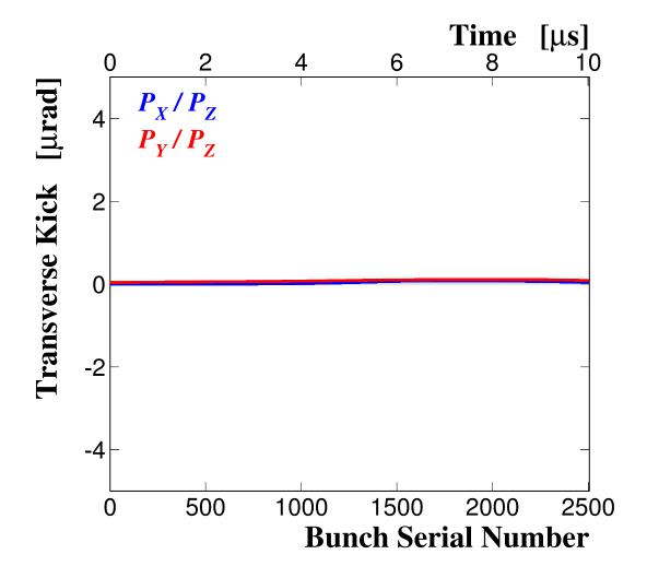
Numerical noise level in the PIC simulation: ≤ 0.1µrad
