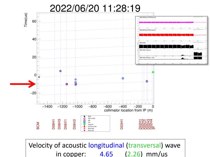
This data suggests that the particle shower produced at the collimator head generated widespread acoustic wave in the downstream of the head, which propagated upstream.
