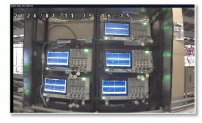
Oscilloscopes should be put near the collimators because of the small analog signals from the acoustic sensors (~0.1 mV at min.)
