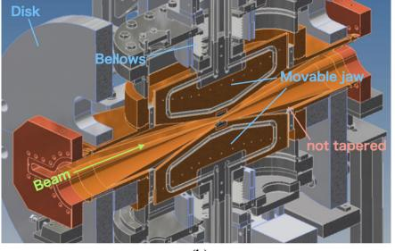
For details of the collimators, refer to "T. Ishibashi et al. Phys. Rev. Accel. Beams 23, 053501 (2020)"
