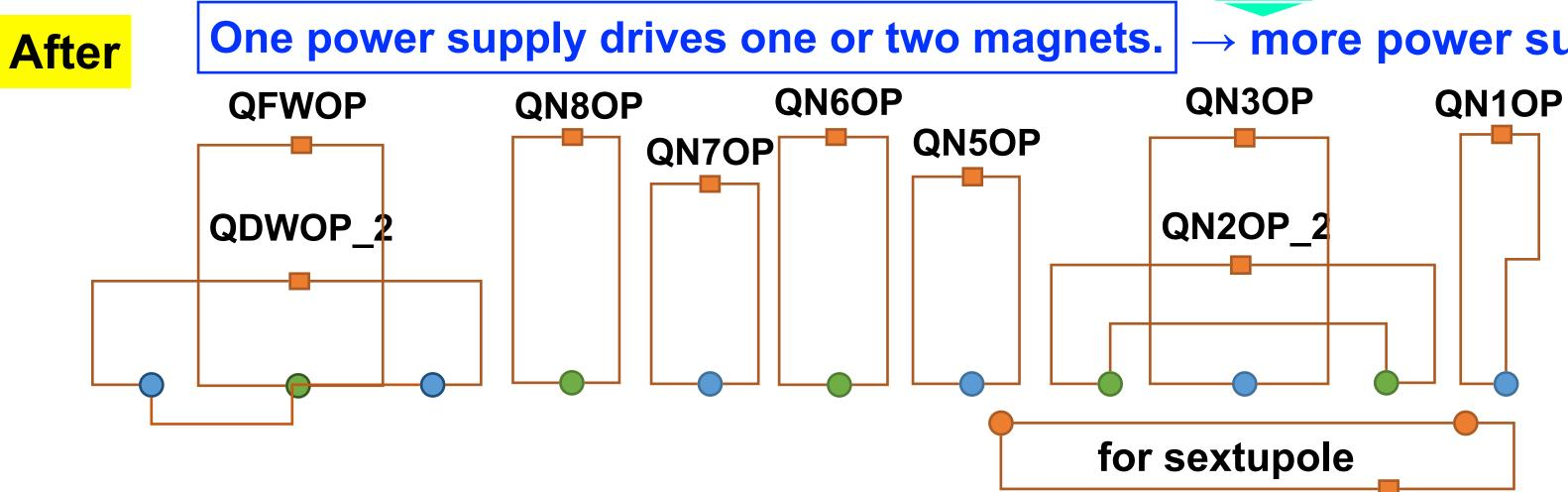
Additionally new power supplies will be installed in September, and test operation of them will start in October. Re-wiring works between the power supplies and magnets has done.
