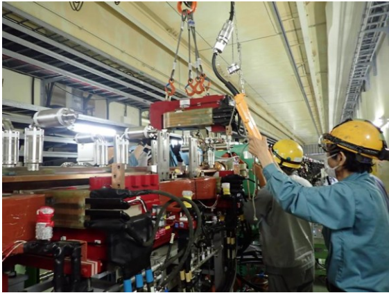
Wiggler magnet disassembly
