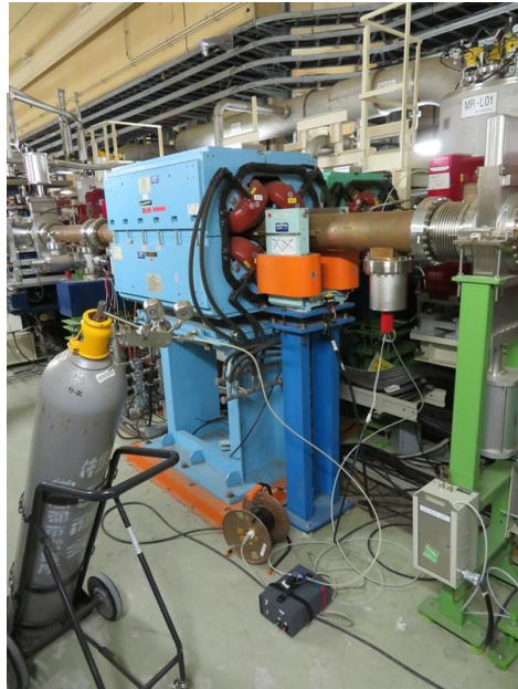
Knocker (driven by compressed air)
