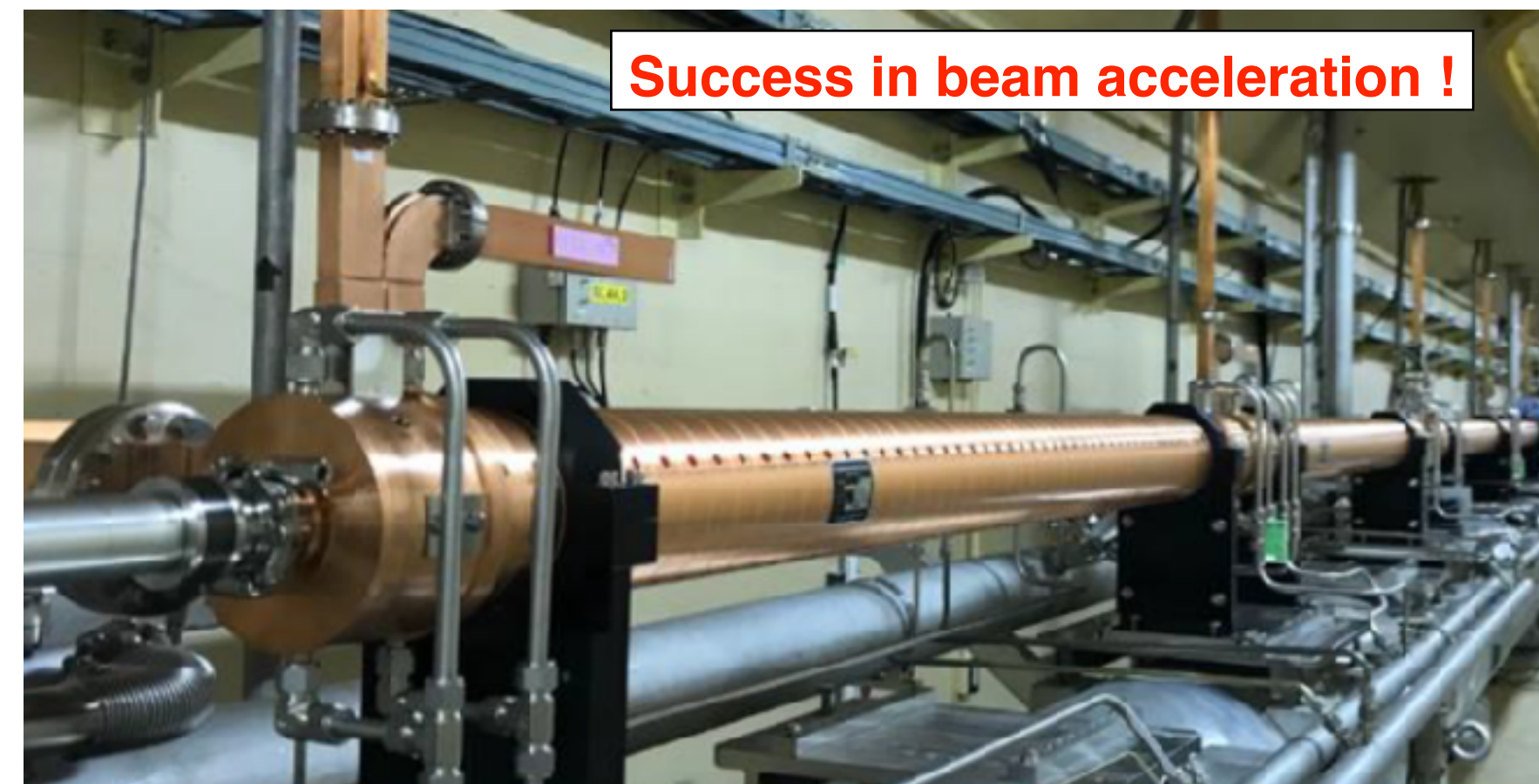
New S-band 2m-long TW accelerating structure
