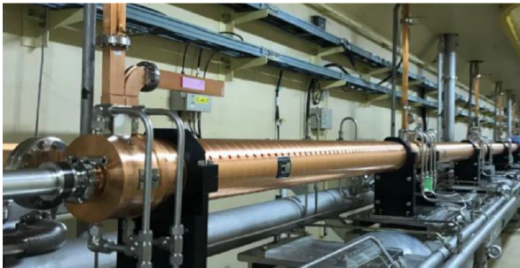
New S-band 2-m-long TW acc. structure
