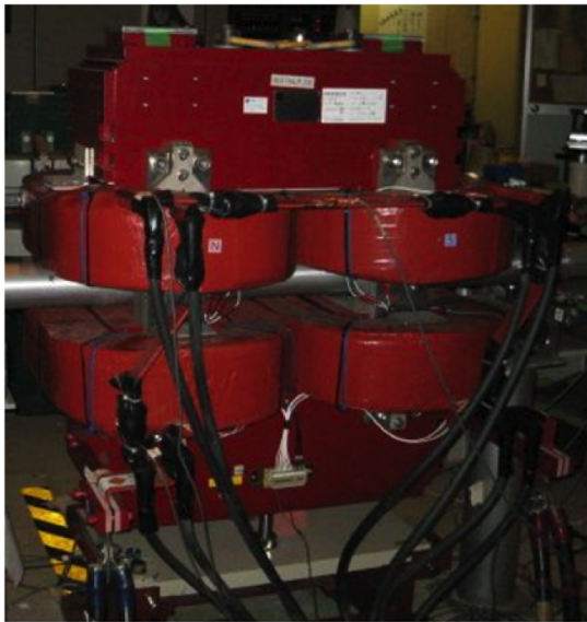
Figure 7.4: Left: Picture of double-pole wiggler magnet "kekB wiggler". Right: Field strength for left and right poles calculated by OPERA-3D.
