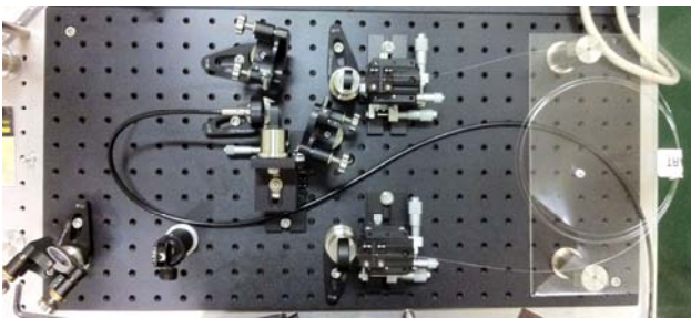
Figure 7: Layout of fiber main amplifier.
