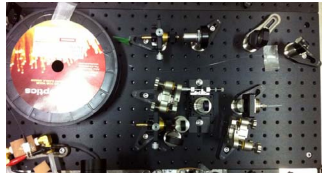
Figure 5: Layout of pre-amplifier.
