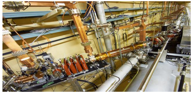
Figure 9: RF-gun studies underway downstream of linac.
