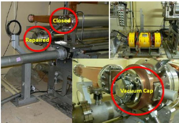
Figure 8: Beamlines are not yet connected (upstream).
