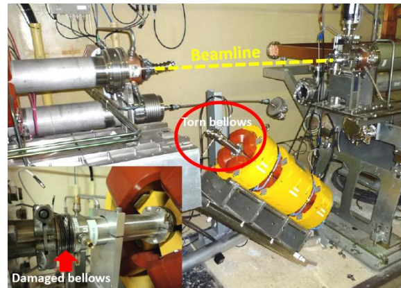
Figure 1: The linac damage in accelerator tunnel.
