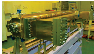
Figure 3: Prototype L-band accelerator structure for BCS.
