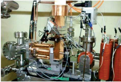
Figure 2: RF gun system installed at 3-2 section.
