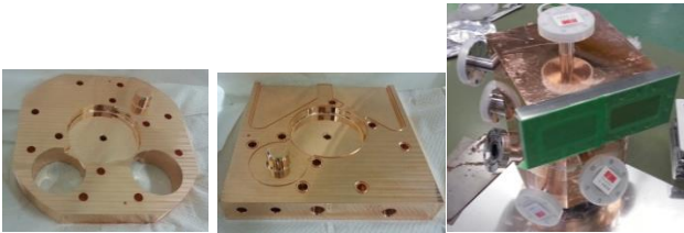
Figure 7: Photo of manufactured cells after brazing.
