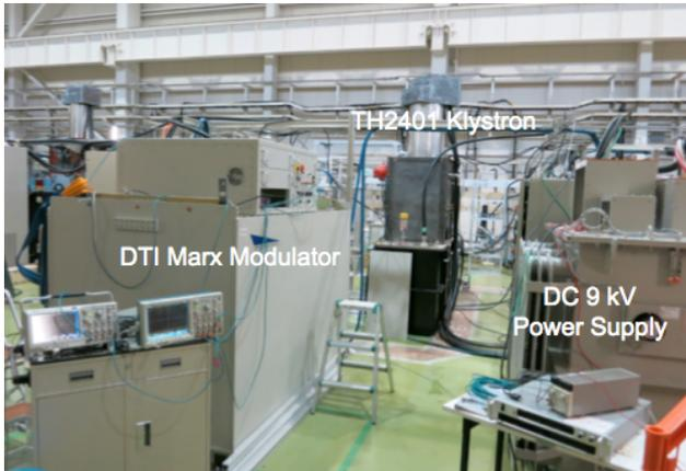
Figure 4: Photograph of STF test stand.
