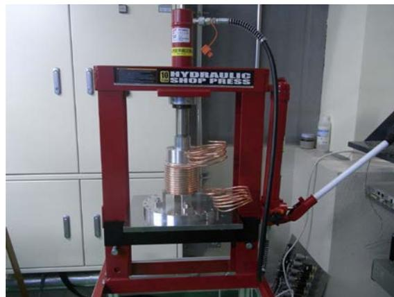
Figure 7: The FC head was pressed by a hand press machine.
