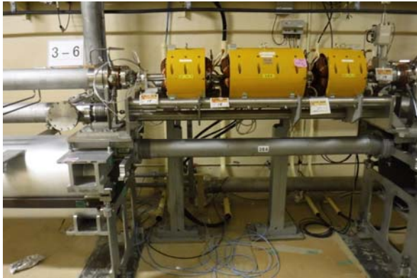
Figure 4: Photograph of the existing DC quadrupole triplet.
