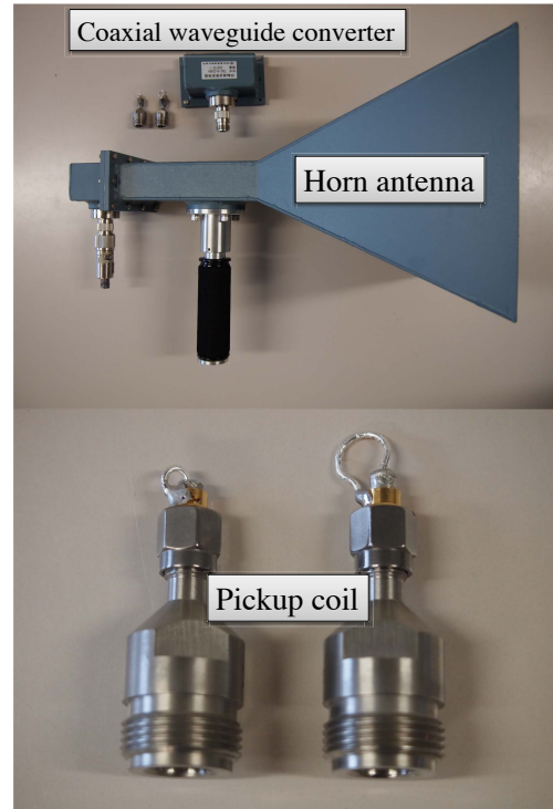
Figure 3: Coaxial waveguide converter, Horn antenna & Pickup coil .
