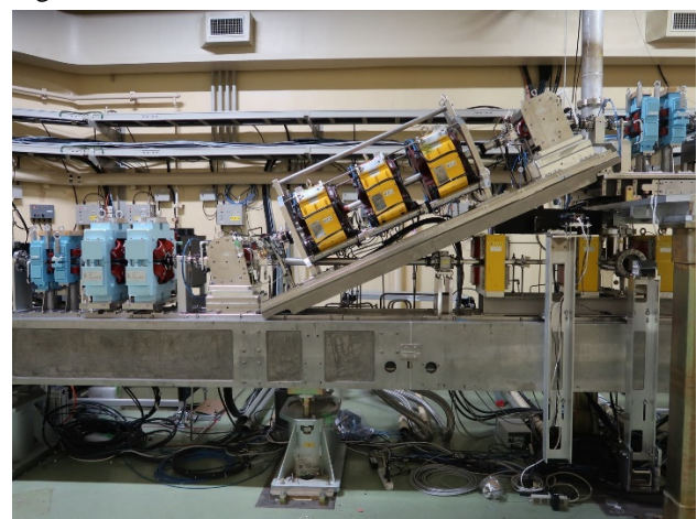
Figure 7: Pulsed magnets at the merge point of A-Sector.
