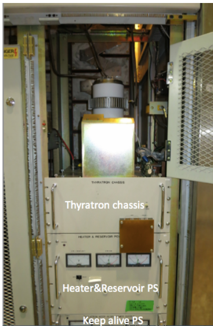
Figure 2: Thyatron switch tube installed in modulator.
