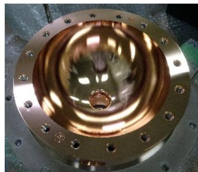
Figure 9: Medium-machined hemisphere with a coupling hole.
