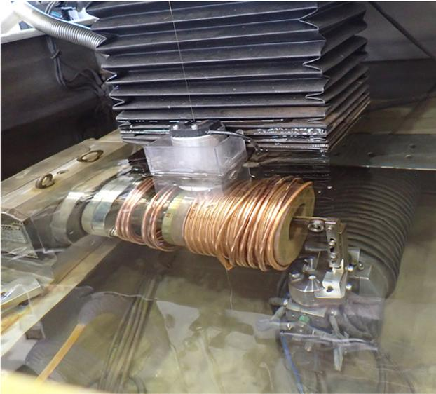
Figure 7: Wire Electric Discharge Machining of the FC.
