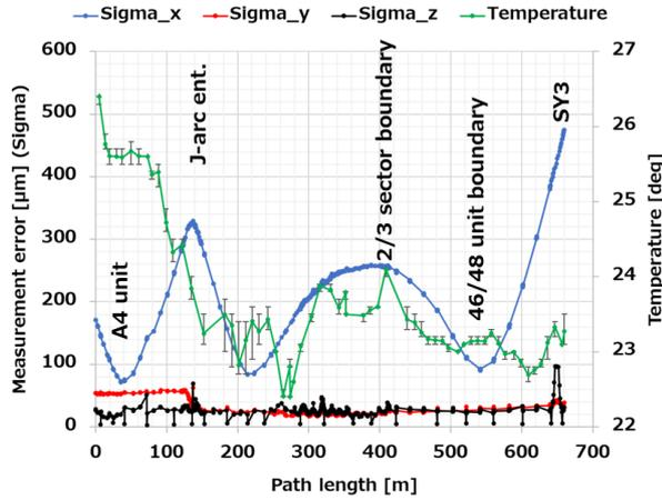
Figure 4: Evaluated measurement errors ( $\sigma$ ) for horizontal coordinates ( $x$ : blue and  $y$ : red) and levels ( $z$ : black) of injector magnets. Room temperature distributions (green) are also overlaid.
