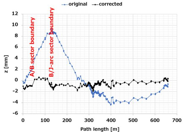
Figure 6: Measured magnet levels along path length before (blue) and after (black) the geoid height correction.
