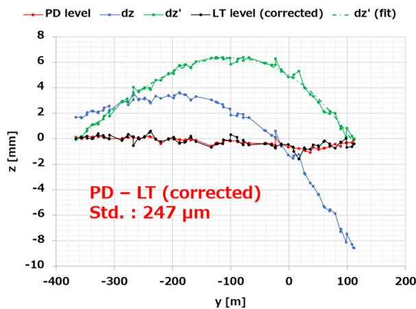
Figure 5: Level survey comparison between PD and LT measurements. Residuals of PD (red) and original LT level data are shown as  $dz$  (blue). Pitching correction of  $20\ \mu\text{rad}$  is applied for  $dz$  data to make even levels of both end with PD levels and plotted as  $dz'$  (green). Eventually, a geoid height correction ( $dz'$  (fit)) is added to the original LT levels (black) and compared with PD level.
