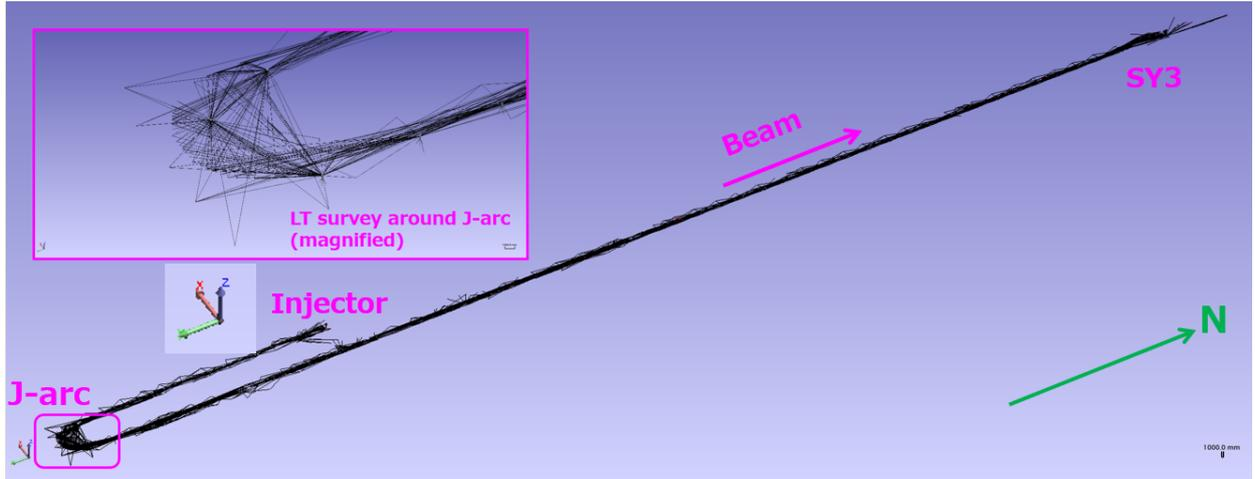
Figure 2: Schematics of the network survey for KEK  $e^+/e^-$  injector linac. A cartesian coordinates are defined with the origin at A sector head.  $y$  and  $z$  axes are beam running and vertical directions, respectively. Note that the beam running direction with this coordinates definition is changed to be negative from exit of the arc section.
