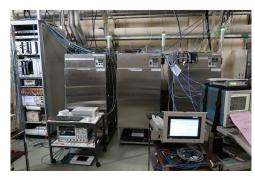
With the upgrade to SuperKEKB, three new phase controllers, MOFB, MOPS, and SECT35PS, were introduced for the linac RF
