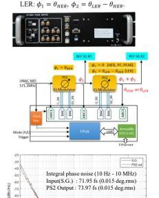
Single sideband (SSB) phase noise of MO phase shifter
