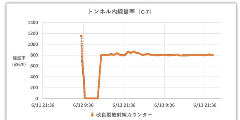
Figure 6: Time traces of the radiation dose rates measured by an improved radiation counter at C-7 during operation and shutdown of the KEK injector linac.
