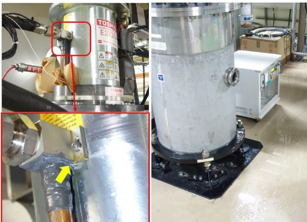
Figure 3: Klystron (C3) water leakage point.
