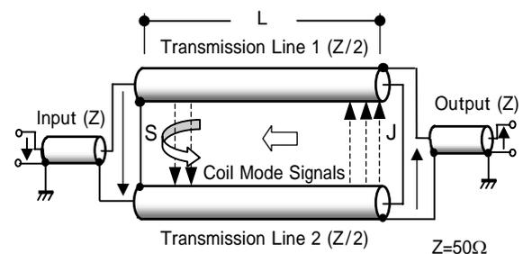
Fig.1. The basis of the structure of the TLBT.
