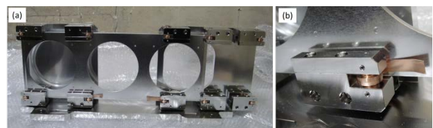
Figure 4: (a) A Frame guide attached a sliding-triple-target frame, (b) gaps between cam-followers and the frame were adjusted by using a 150 μm thickness tape.
