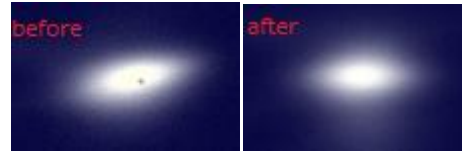
Figure 11: Beam image measured by a CCD camera after revision of vertical dispersion it with before revision.
