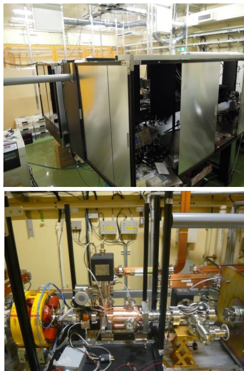
Figure 4: A1 laser room (upper) and Disk and Washer type photocathode RF Gun(lower).
