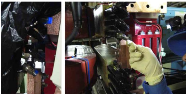
Figure 6: Black light examination (left) and rinsing of the hose connection.
