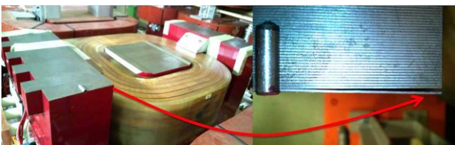
Figure 9: The laminate sheet peeled off from the wiggler magnet core.
