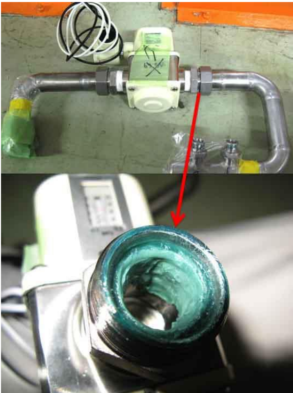
Figure 2: The location where the green object was found (top) and the contamination found inside (bottom).
