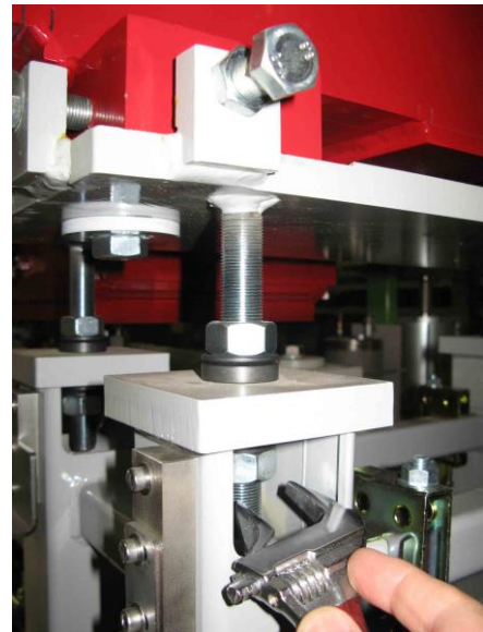
Figure 10: A wrench for turning a screw for adjusting the magnet height barely fits in the space.
