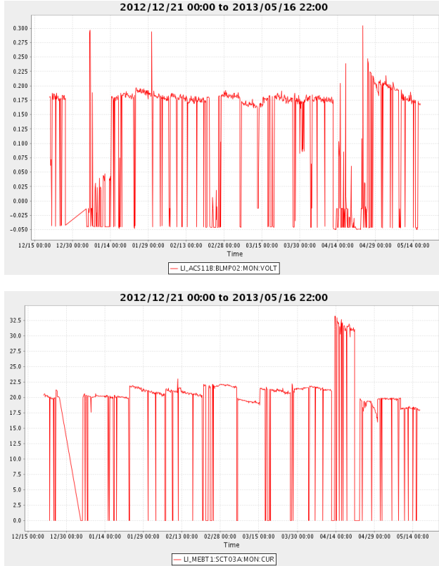
Figure 2: Top: The beam loss pulse amplitude as a function of the date measured by a proportional counter at ACS11. Bottom: The peak beam current (mA) as a function of the date at the upstream of MEBT1.
