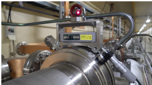
Figure 3: Measurement tool of accelerator tube for laser tracker.
