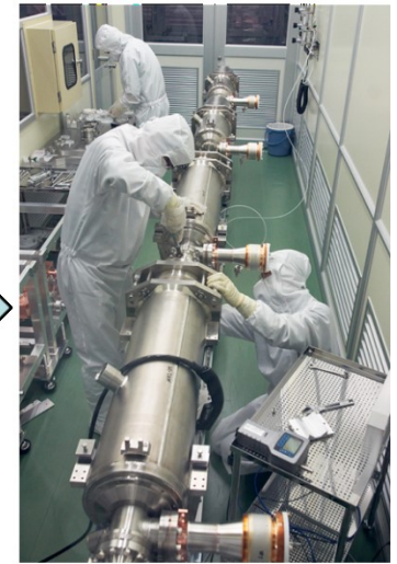
Cavity unit with Jacket at 1.25 times of design pressure (test with He gas : 0.25 MPa)
