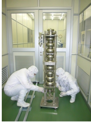
Assembly (Class 10) Baking (120°C, 48h) Hanging stand with T-map (Class 1000)
