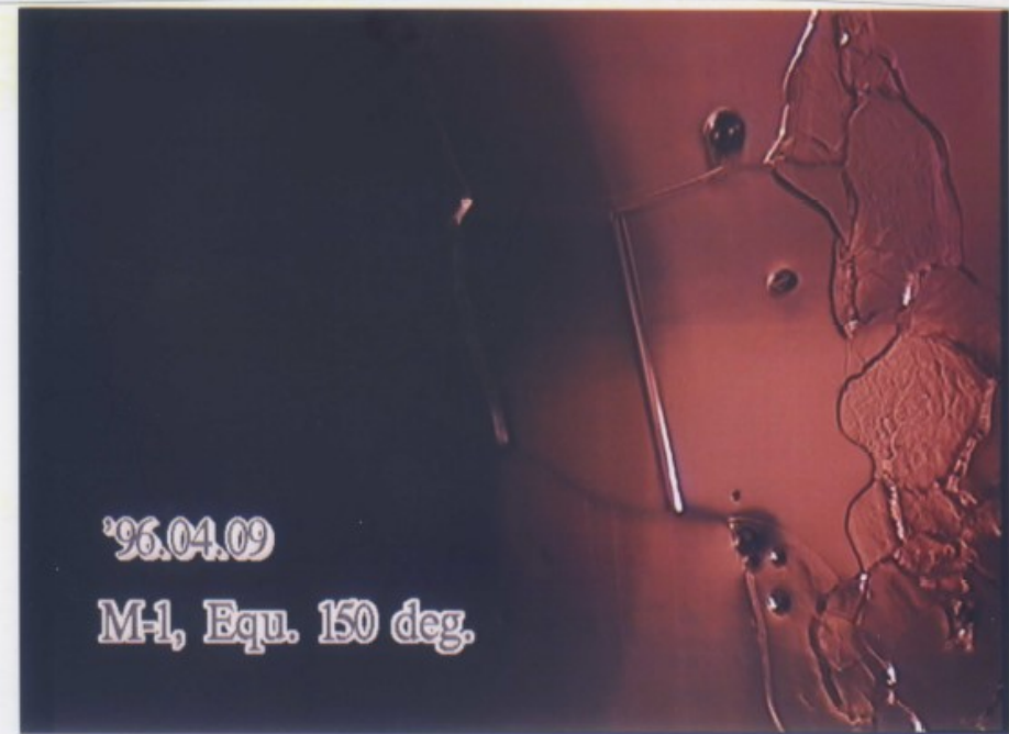
M - 1 Cavity ; Quench Location (EBW seam at Equator)
