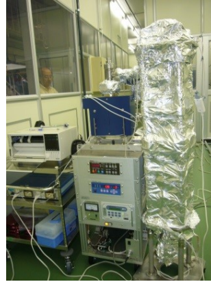
Assembly (Class 10) Baking (120°C, 48h) Hanging stand with T-map (Class 1000)
