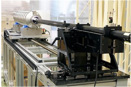
Inspection of inner surface
