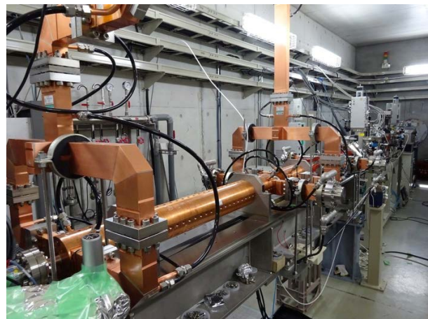
Figure 3: Accelerator structures with double-feed waveguide coupler.
