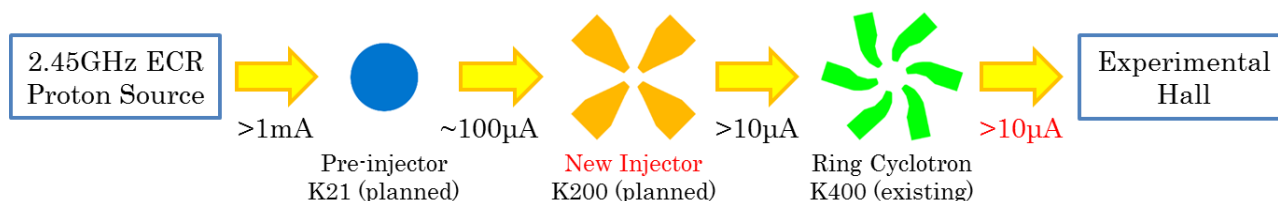
Figure 2: New cyclotron cascade under contemplation.
