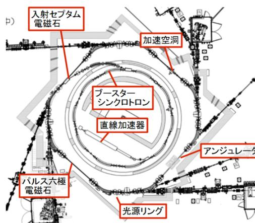
Figure 1: Accelerator complex of Aichi SR.
