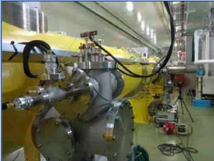
Conduction cooled quadrupole magnet was fabricated by FNAL, installed into CM-1 at STF.
