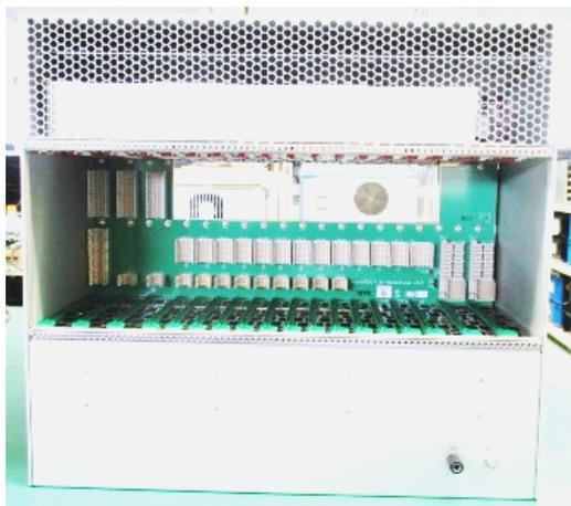
Figure 5: MTCA.4 shelf with RF backplane (rear view).
