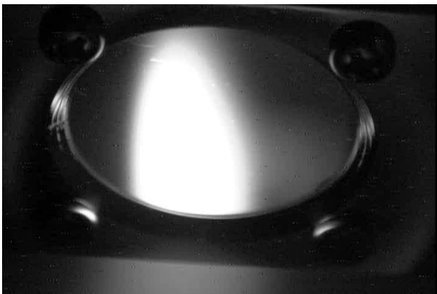
Figure 4: Beam profile measured with a YAG screen monitor. The screen size is 23 mm in diameter.
