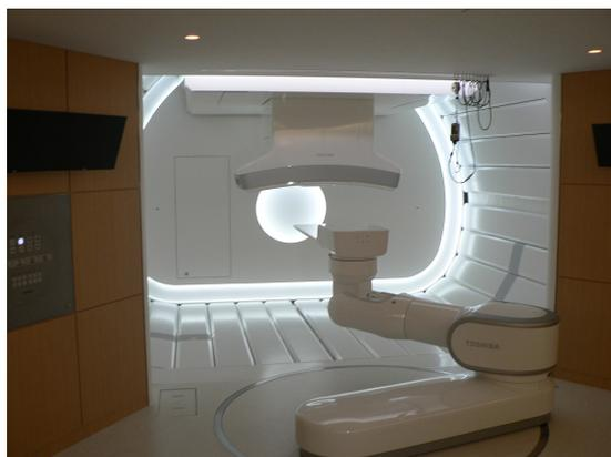
Figure 7: Photograph of covered nozzle and treatment room for rotating gantry.
